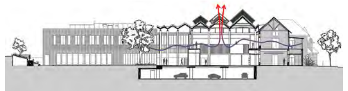
Figure 20. Diagram of natural air movement through the main spaces of the library. (Image: BVN)
