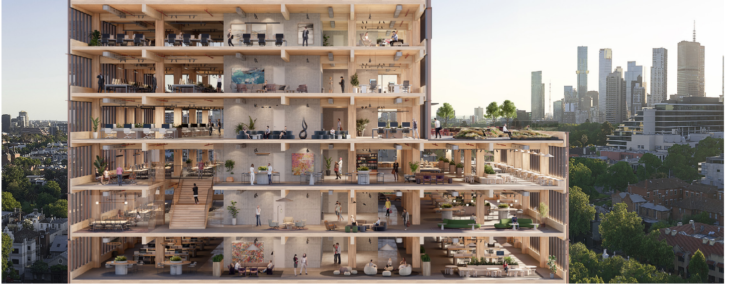
Figure 10. Diagrammatic render, column beam and CLT slab with central concrete stability core. (Image: Hines)
